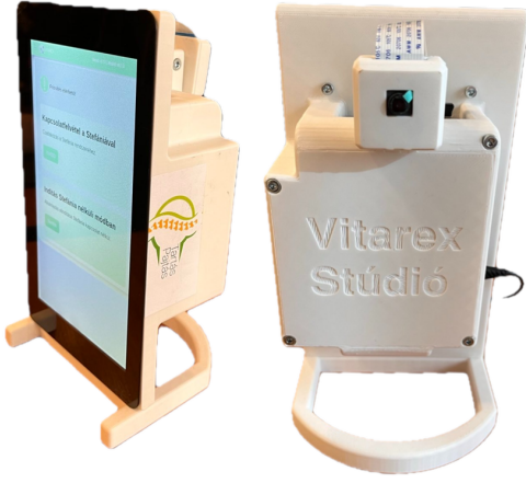
Fig. 1: Two photos of the Posture Buddy device.
